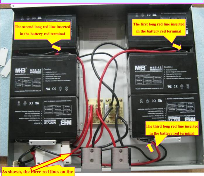
As shown, the three red lines on the switch needs up to the external connector below.
